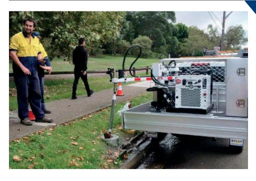
The Compact VMS, an E.H. Wachs exclusive valve maintenance skid, comes with our industry-leading ERV-750 extended reach valve exerciser, our newest controller - the HC-100 handheld computer/controller/datalogger with GPS and VITALS software.
